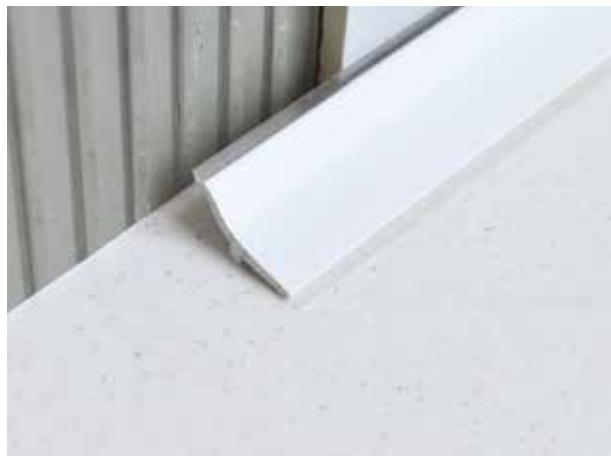
Hygienic cove shaped profile between wall and wall and between wall and floor. Connections between the wall and the bathtub, the shower tray or the kitchen surface. The silicones that are normally used lose their anti-mold properties after few months producing unsightly halos or stains. SB24 is easily applied with FIXXTEC on coverings, improves or restores the appearance of corners, making them more hygienic.
